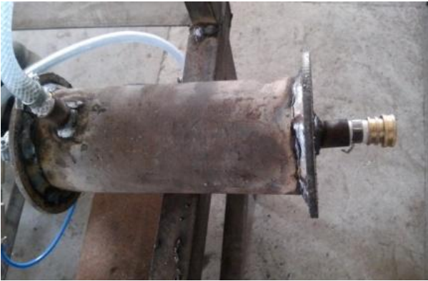
Fig 2. Heat exchanger setup
